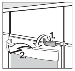
The lock is fitted beneath the control panel to prevent the door from being opened. The door can only then be opened by pressing the lever.
